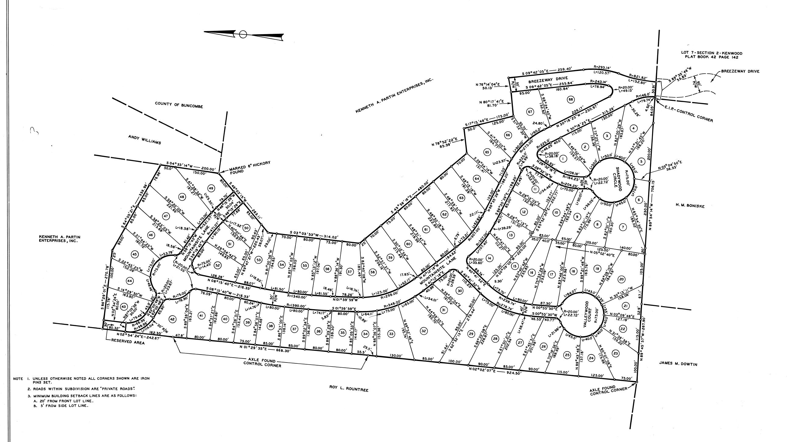
I, KENNETH T. MILLS CERTIFY THAT UNDER MY DIRECTION SEAL AND SUPERVISION THIS MAP WAS DRAWN FROM AN ACTUAL FIELD LAND SURVEY; THAT THE ERROR OF CLOSURE AS CALCULATED BY LATITUDES AND DEPARTURES DOES NOT EXCEED 1:10,000; THAT THIS MAP WAS PREPARED IN ACCORDANCE WITH G.S. 47-30 AS AMENDED.
