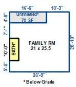
Bath\* (41 sf) is finished but has no heat It does not meet the 7' ceiling height requirement. It is not included in the finished basement total.
